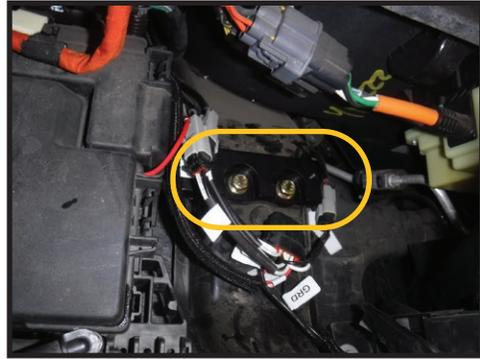
**4. Mount the IIC to the IIC mount using the supplied 1/4" hardware(PN 605069). Use a 7/16" to tighten. Insert the block off plug into the grey port of the IIC. Insert the main wire harness into the black port of the IIC. [FIGURE 6 & 7]**
