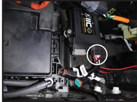
**5. Route the 2 black (Ground) wires to the ground location on the passenger fender. Cut to length, strip, and crimp the terminal connectors (PN 605751) on. Use a heat gun to activate heat shrink. Fasten the terminal connectors to the fender ground using an 8mm. [FIGURE 8]**
