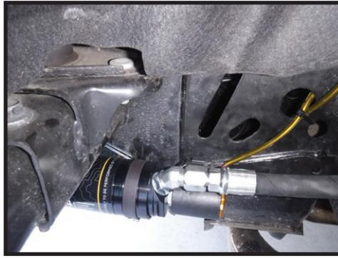
**17.** Route the 20-FT and 26-FT wires across to the driver front wheel well. Route the wires down the back side of the wheel well to the body mount. Route the wires along the factory wire harness.
