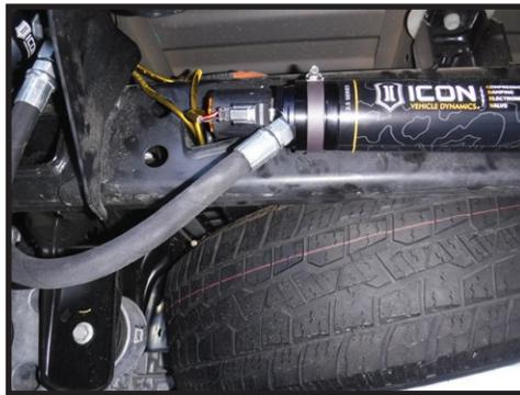
**20.** Route the 26-FT wire along the crossmember to the passenger rear wheel well. Connect the wire the solenoid on the shock. [FIGURE 15]
