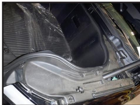
**2. Remove the battery access panel. [FIGURE 3]**
